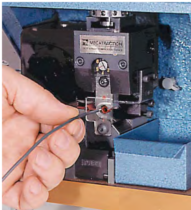
Insert the conductor into the terminal or disconnect.
