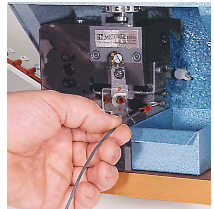
Next terminal or disconnect is automatically positioned under the dies.
