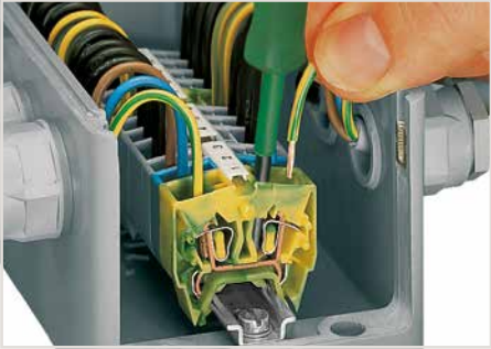
CAGE CLAMP® connection Inserting a conductor. With ferruled conductors, it is necessary to use a terminal block one size smaller than the conductor's nominal cross section.
