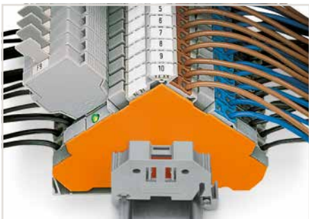
The fuse plug is 1 mm wider than the terminal block, so an intermediate plate must be installed.
