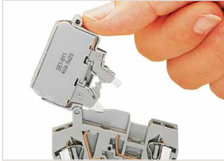
Fuse replacement: Before replacing a fuse, pivot the fuse holder into the locked open position.
