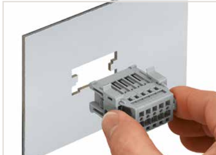
Insert male connector with snap-in flanges (769-605/006-000) into the cutout.
