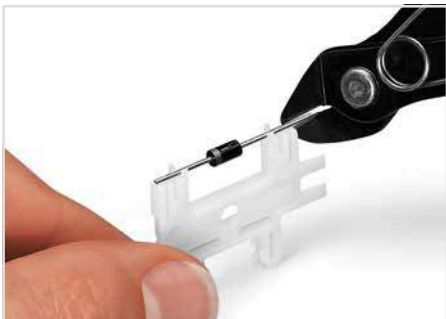
Cutting component to the proper length.
