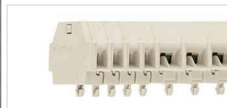
Terminal strip with snap-in mounting feet, for 0.6 ... 1.2 mm plate thickness, 3.5 mm mounting hole diameter (also for 210-154 Aluminum Rail or with 209-120 Mounting Foot for DIN-35 rail)
