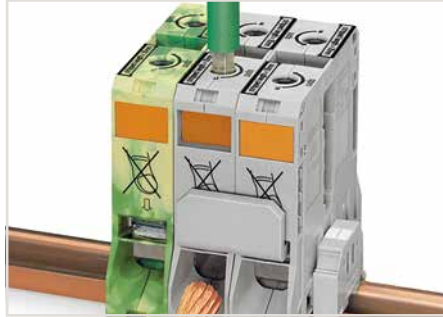
Conductor termination – step 2 Insert a stripped conductor into the clamping unit until it hits backstop. Hold in this position.
