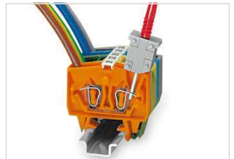
Testing via CAGE CLAMP® on the current bar (max. nominal current: 6 A). CAGE CLAMP® clamps individual test contacts. The maximum test voltage is 400 V.
