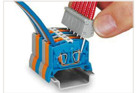
Testing by touch contact to the CAGE CLAMP® spring (limited to 0.5 A and 48 V test voltage) – test pins are not protected against accidental contact.
