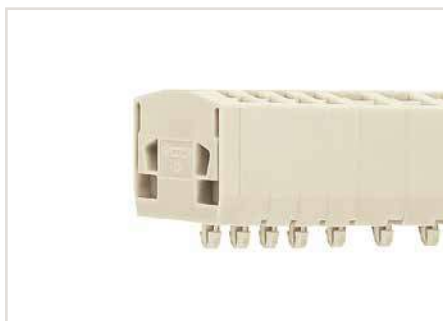
Terminal strip with snap-in mounting feet, for plate thickness 0.6 mm ... 1.2 mm, fixing hole 3.5 mm Ø.
