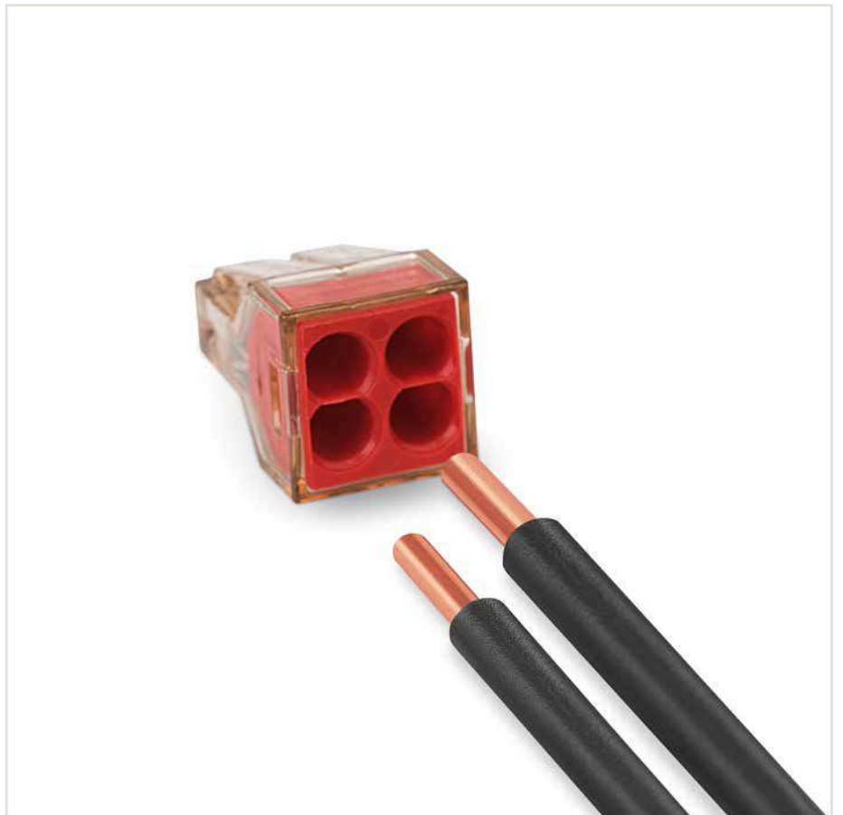
Removal: Hold conductor to be removed and twist alternately left and right while pulling the connector.
