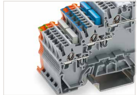
Ground commoning: For sensor and actuator terminal blocks without ground connection to the DIN-rail, the ground connection can be performed by commoning to the terminal block with a ground foot.
