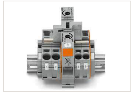
Commoning 35 mm 2 (2 AWG) POWER CAGE CLAMP Terminal Blocks with 10/16 mm 2 (8/6 AWG) 2010 and 2016 Series TOPJOB® S Terminal Blocks using step-down jumpers (not valid for 2016-76xx and 2016-77xx).
