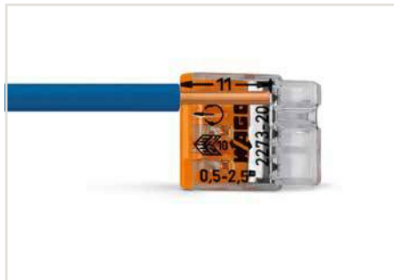
Strip solid conductor to 11 mm / 0.43 inch (see marking).
