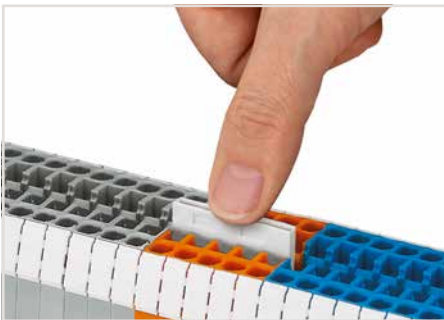
7 Push jumper bars down firmly until fully inserted. When using multipole bars, push alternately on the right and then left side, until installed. Push-in type jumper bars 1 - 3 - 5 - 7 or 1 - - 4 - - 7 upon request
