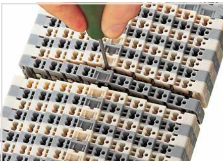
Open the assembly by laterally sliding a block via operating tool (2.5 x 0.4 mm blade).
