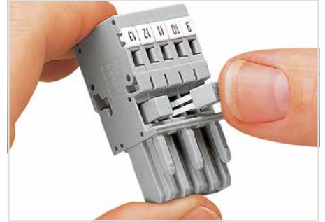
Commoning 1-conductor female plugs via miniature adjacent jumpers.
