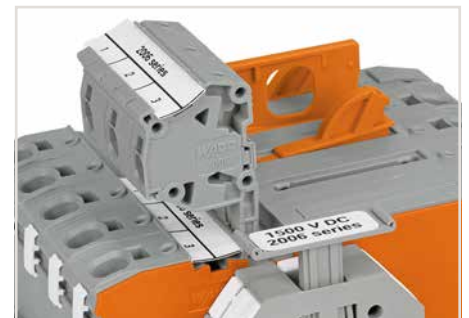
Alternatively, measurement can also be performed using TOPJOB® S Connectors (2006-511) from terminal block 1 to 2. Spacer modules (2006-549) must be used to compensate for the 15 mm terminal block width.
