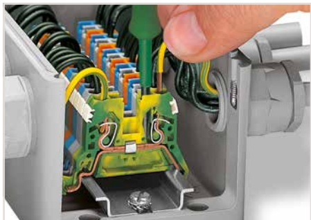
CAGE CLAMP® connection Inserting a conductor (0.08 ... 4 mm² "f-st"). With ferruled conductors, it is necessary to use a terminal block one size smaller than the conductor's nominal cross section.
