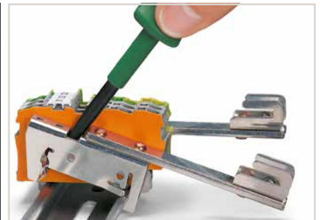
Remove the busbar carrier using an operating tool (type 3, 5.5 x 0.8 mm blade).
