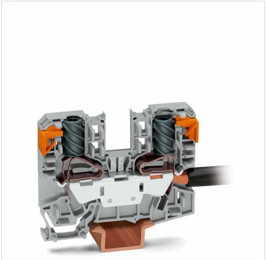
Conductor termination – step 3 A small counter-clockwise rotation closes the clamp, securing conductor ①. When unlocked, allow operating tool to rotate clockwise ② to securely terminate the conductor.
