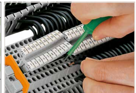
The flexible marker carrier, which is placed above the wiring level, can be pushed aside during wiring or commoning. The carrier has two staggered levels for WMB markers that perfectly align with the terminal block decks.
