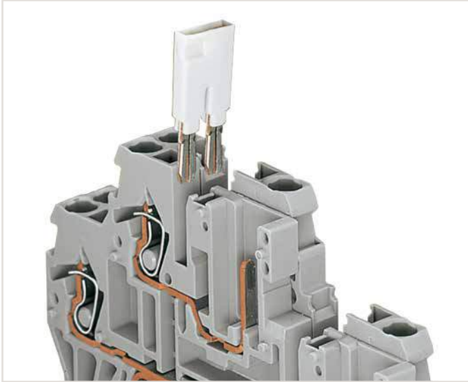
Commoning a double-deck through terminal block (870-501) with a 1-conductor/1-pin double-deck terminal block (870-101) via push-in type jumper bar.
