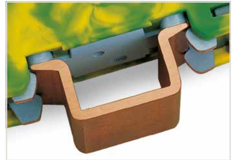
Grounding foot Ground conductor terminal blocks (limited to max. 120 mm 2 /250 kcmil per EN 60947-7-2) must be snapped onto a 2.3 mm thick copper carrier rail.
