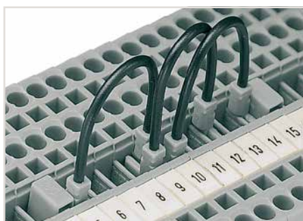
Compared with the 279 Series, the 280/775/780 and 281/776/777/781 Series can also accommodate two wire jumpers, allowing the use of commoning chains. Furthermore, the 280/769/775/780/880 and 281/776/777/781 Series allow both wire jumper and adjacent jumper to be simultaneously plugged into a same terminal block.
