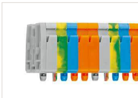
Terminal strips with snap-in mounting feet, for 0.6 ... 1.2 mm plate thickness, mounting holes: 3.5 +0.1 mm Ø
