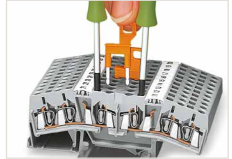
Using terminal blocks for matrix patching as disconnect terminal blocks via disconnect jumpers.
