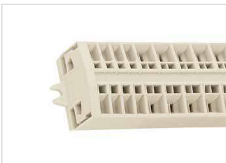
Terminal strip with mounting flanges, for screw or similar mounting types, fixing hole 3.2 mm Ø.
