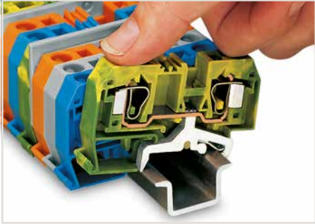
By snapping a ground conductor terminal block onto the carrier rail, a direct electrical connection is automatically made to the rail.
