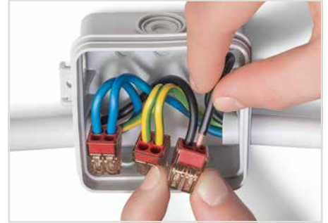
Termination: Insert stripped solid conductor until it hits backstop.
