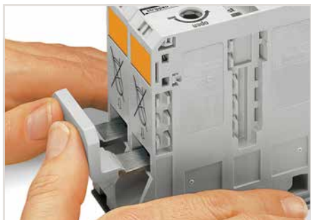
Commoning with an adjacent jumper: Insert the jumper above the conductor entry hole – prior to conductor termination. The nominal cross-section remains unchanged.
