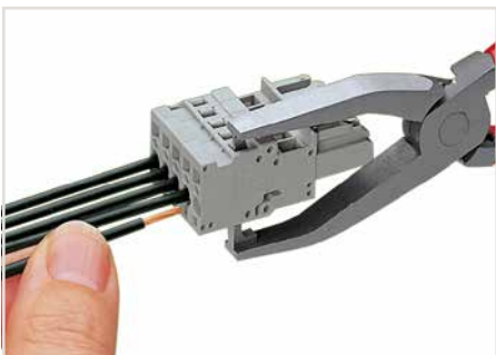
Operating tool Inserting a conductor via operating tool - side-entry wiring (example shows a female plug). With ferruled conductors, it is necessary to use a terminal block one size smaller than the conductor's nominal cross section.
