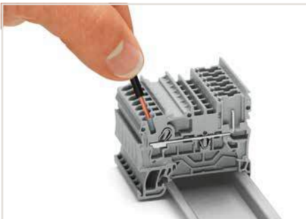
Push-in CAGE CLAMP® enables solid conductors and fine-stranded conductors with ferrules to be connected by simply pushing them into the unit.
