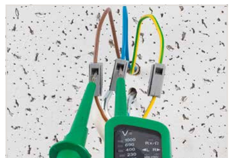
Testing via separate test ports.
