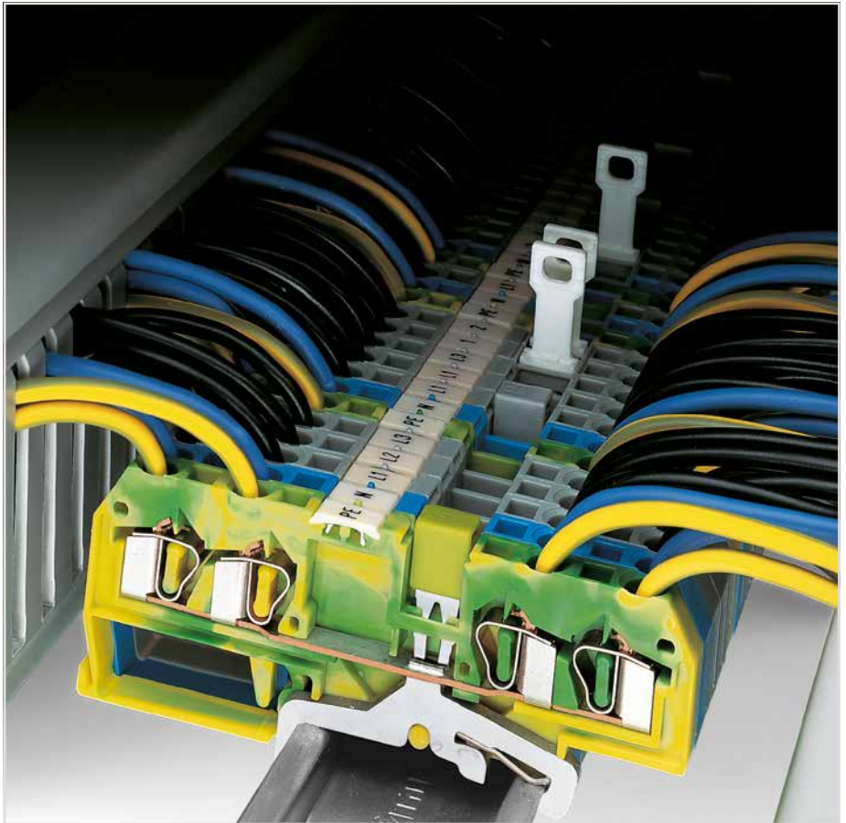
Steel carrier rails are not suited for PEN (ground and N-conductor) applications per EN 60947-7-2 (VDE 0611, Part 3).
