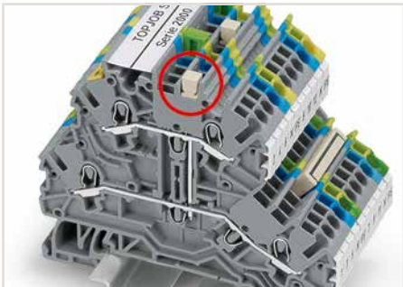
Commoning two levels via double-deck vertical jumper (2000-492).
