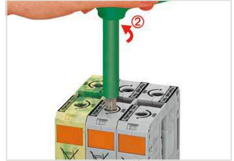
Conductor termination – step 3 A short counter-clockwise rotation ② releases the locking tab. When unlocked, the T-wrench rotates clockwise, securely clamping the conductor.
