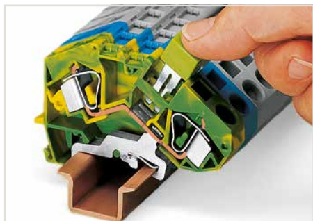
Commoning ground conductor terminal blocks with through terminal blocks is possible in one direction only (via rear side of terminal block) using adjacent jumpers. In addition to the required marking of these blocks, use yellow-green adjacent jumpers.
