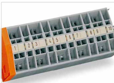
Combining 2- and 4-conductor terminal blocks. Marking via Mini-WSB Quick markers.
