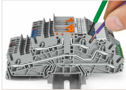
Inserting a conductor via operating tool. Connecting fine-stranded conductors without ferrules, or small cross-sectional conductors that cannot be pushed in, is performed similarly to the original CAGE CLAMP® - just use an operating tool.
