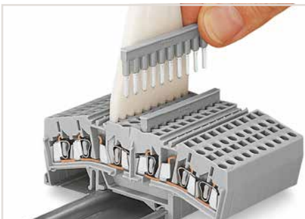
Multiplying potentials via 10-way comb-style jumper bar. (only possible in the terminal block's center)
