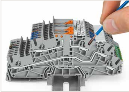
Inserting conductors via push-in termination. Solid conductors with cross-sections from either one size above, or up to two sizes below, the rated cross-section can be simply pushed in - no tools needed.
