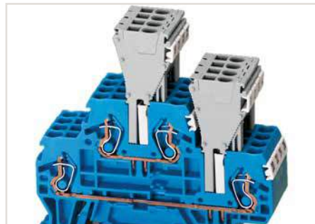
The tap-off module assembly can be directly plugged into the jumper contact slot of the current bar. The terminal blocks can also be commoned via push-in type jumper bars parallel to the jumper slots being used by the modules.
