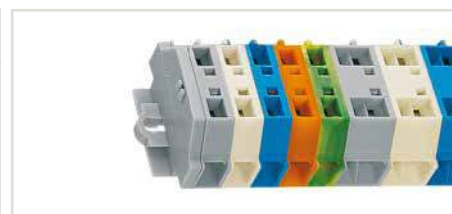
Terminal strip, with mounting flanges, for screw or similar mounting types, 3.2 mm mounting hole diameter (with 209-123 Mounting Foot for DIN-35 rail)
