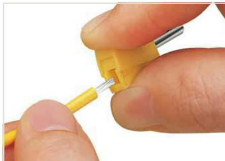
Conductor termination: Press button fully, insert stripped conductor into square entry and release.
