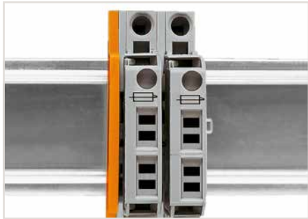
An intermediate plate is supplied with all 10 mm wide fused disconnect terminal blocks. At the end of an assembly or if there is no adjacent fused disconnect terminal block, an end or intermediate plate must be used.
