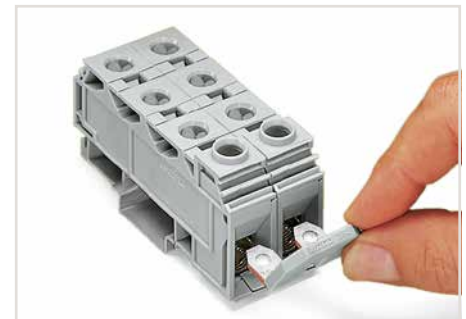
Commoning with comb-style jumper bar. Individual arrangement: 125 A Two jumpers combined in one clamping unit: 100 A
